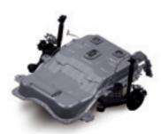
The increased power density of this advanced battery delivers more performance and greater driving range. The battery is located low in the chassis for better handling characteristics. To further improve recharging times the AC onboard charger has been increased to 7.2 kW.
